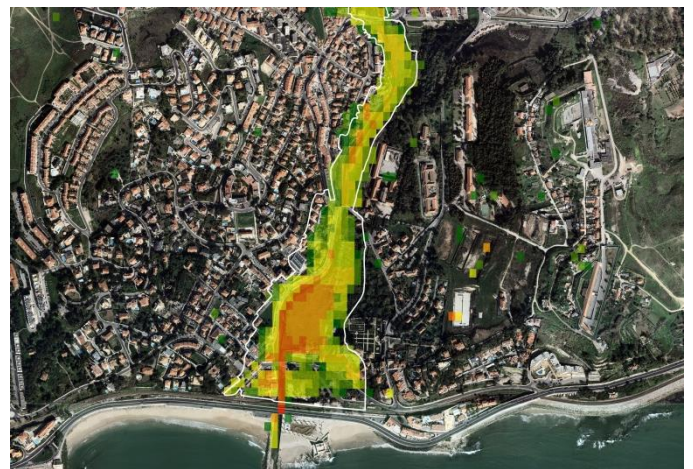
Figure 6. Maximum water depth result for precipitation occurred in 18/2/2008. At white the delimitation of flood areas occurred in 1983. Source: own production
